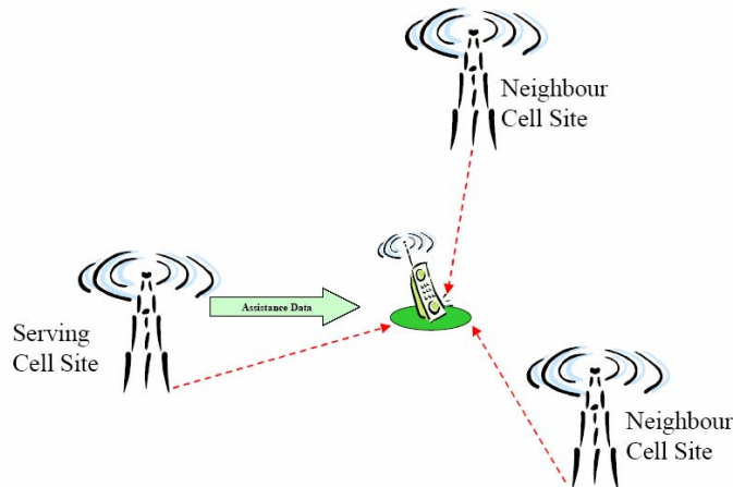
Figure 2-C E-OTD [10] The handset measures the arrival time of signals transmitted from three or more Base Transceiver Stations (BTS), and estimates position using triangulation.
